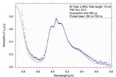
Figure 7. Single shot (17 µs total scan time) transmission data for Freon 134a. HITRAN data were convolved with the measured linewidth of the laser emission (Freon at 2.36% concentration, temperature of 23°C, and pressure of 760 Torr).
