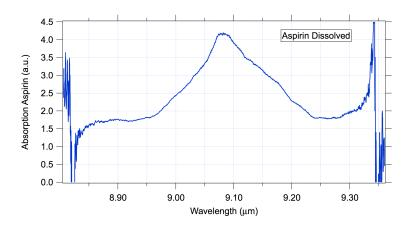
Figure 11. Single shot (1 ms total scan time) standoff detection of aspirin.
