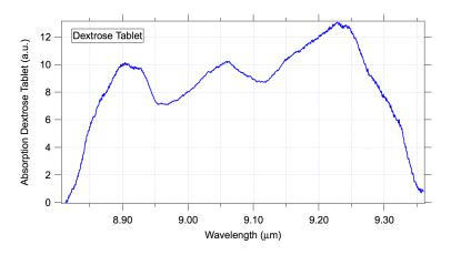
Figure 9. Single shot (1 ms total scan time) standoff detection of dextrose tablet.
