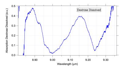
Figure 10. Single shot (1 ms total scan time) standoff detection of dissolved dextrose.
