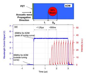
Figure 6. Switching time measurements of AOM tuned QCL. Top panel shows the geometry of the AOM. Panel (a) shows the details of laser turn on when the AOM frequency is changed from 35 MHz (outside the range of AOM tuned QCL operation) to 45 MHz (peak power wavelength for the AOM tuned QCL as seen from either Figure 2 or Figure 4)
