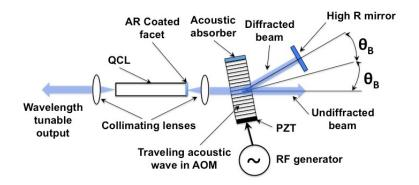
Figure 1. Schematic of a travelling wave acousto-optic modulator tuned quantum cascade laser in Littrow configuration [1]
