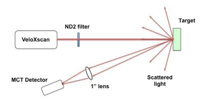
Figure 8. Experimental setup for standoff detection demonstration.
