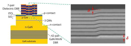
Figure 7. (Left) A schematic illustration of a GaN-based VCSEL structure having a dielectric current aperture. (Right) A scanning electron microscope (SEM) image of a structure with a depression  $\delta$  in the center: Note that  $\delta$  is the same as the dielectric layer thickness indicated at bottom right in the figure.
