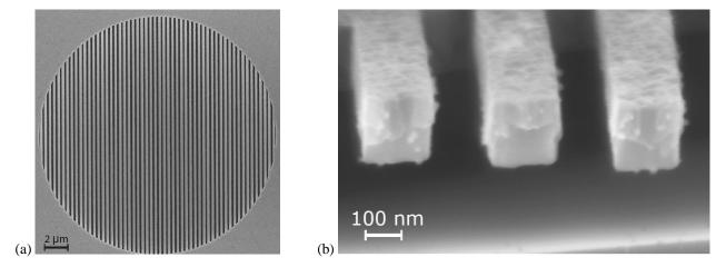
Figure 12. SEM image of a free-standing TiO<sub>2</sub> HCGs with a period of 350 nm and duty-cycle of about 50% in (a) top view and (b) cross-sectional view.
