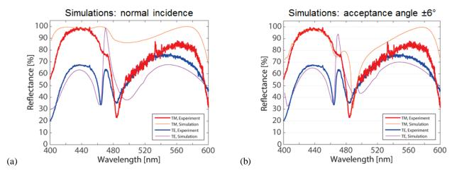
Figure 13. Measured reflectance spectra of the TiO<sub>2</sub> HCG with a period of 370 nm, a duty cycle of about 45%, a grating layer thickness of 210 nm and an airgap of 340 nm, for both TM and TE polarized light, and (a) simulations assuming only normally incident light and (b) simulations accounting for a finite acceptance angle of 6°.
