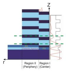
Figure 8. Schematic illustration of a part of the VCSEL structure where the introduction of an aperture has resulted in a depression in the central region. At the cross-sections shown by green dashed-lines the refractive index is lower in the center compared to the periphery, which can possibly lead to antiguiding. Also shown is the refractive index profile along the center of the device and the amplitude of the optical field along the symmetry (z-) axis.
