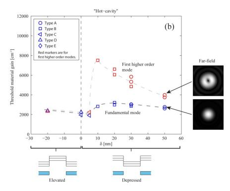
Figure 9. Threshold material gain in the QWs for of the fundamental and first higher order modes. The marker type indicates the type of current aperture, specified in Ref.<sup>132</sup> (a) for cold-cavities, and (b) for hot cavities when thermal lensing is included. Insets show the cross-section of the laser beam in the far field from the indicated VCSELs.
