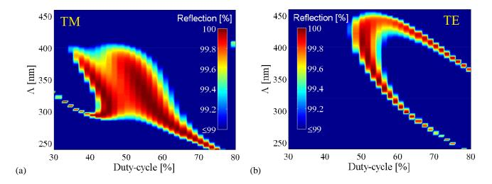
Figure 11. The reflectance contour plots (reflectivities above 99%) for  $TiO_2$ /air HCG using the optimal layer thickness values for (a) TE-polarized light,  $TiO_2$  layer thickness  $t_g = 145$  nm, airgap height  $h_a = 550$  nm, and (b) TM-polarized light,  $t_g = 205$  nm,  $h_a = 400$  nm.
