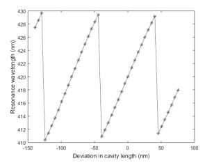
Figure 5. Threshold material gain and resonance wavelength as a function of a deviation in cavity length (n-GaN thickness) for a GaN-VCSEL with a 7-pair TiO<sub>2</sub>/SiO<sub>2</sub> DBR on top and an epitaxial 42-pair AlInN/GaN as the bottom DBR.
