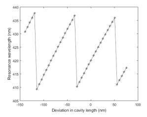
Figure 4. Threshold material gain and resonance wavelength as a function of a deviation in cavity length (n-GaN thickness) for a GaN-VCSEL with a 7-pair TiO<sub>2</sub>/SiO<sub>2</sub> DBR as the outcoupling DBR and 11-pair TiO<sub>2</sub>/SiO<sub>2</sub> DBR as the highly reflective DBR.
