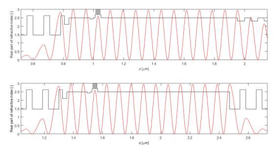
Figure 3. Standing optical wave inside the cavity for a GaN-VCSEL with an outcoupling DBR of 7-pairs of  $TiO_2/SiO_2$  and a highly reflective DBR of 42-pairs of AlInN/GaN (top figure) and 11-pair  $TiO_2/SiO_2$  (bottom figure).
