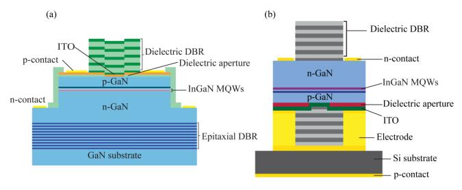
Figure 2. A schematic view of a GaN-based VCSEL with (a) one epitaxial and one dielectric DBR and (b) two dielectric DBRs.
