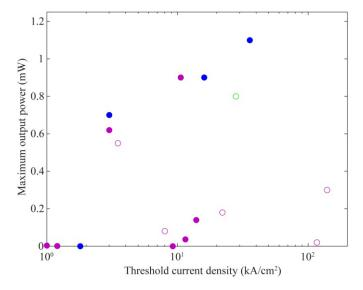
Figure 1. Optical output power and current density for electrically injected GaN-VCSELs published to date.  $^{27-30,32-47}$  Filled markers illustrate continuous wave operation and open markers pulsed operation. The colors indicate the lasing wavelength, violet (406 nm - 422 nm), blue (446 nm - 463 nm), and green (503 nm).
