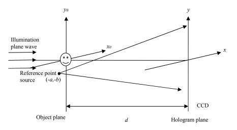
Fig. 1 Schematic diagram of Lensless Fourier transform digital holography
