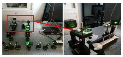
Fig. 3 Lensless Fourier digital holographic experiment setup
