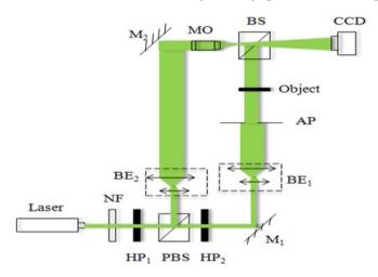
Fig. 2 The schematic of the lensless Fourier digital holography
