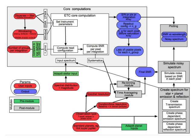
Figure 4. Flow chart representation of the main NEETC modules.
