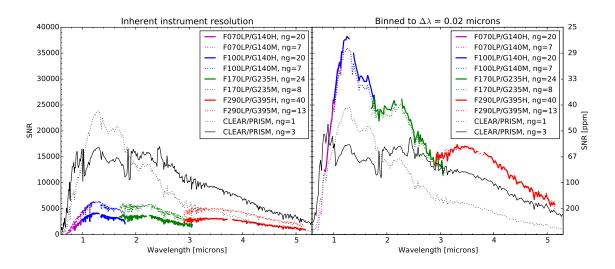
Figure 7. SNR obtainable for GJ1214 for all 9 instrument configurations for one transit (52 min). Left panel shows SNR for the inherent instrument resolution and right panel the SNR binned to a uniform dispersion of  $\Delta \lambda = 0.02 \ \mu m$ .
