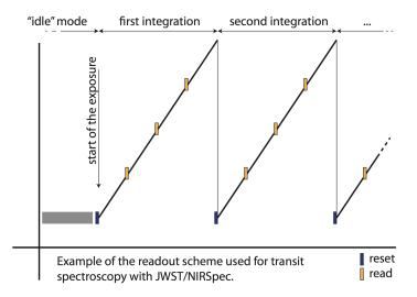
Figure 2. Illustration of the specific MULTIACCUM readout scheme used by NIRSpec when observing transiting exoplanets. In this example an individual integration consists of a reset followed by 3 groups each containing one frame. The exposure contains multiple integrations. The detector duty cycle is 75% as one forth of each integration is used to reset the detector. Figure from [8].
