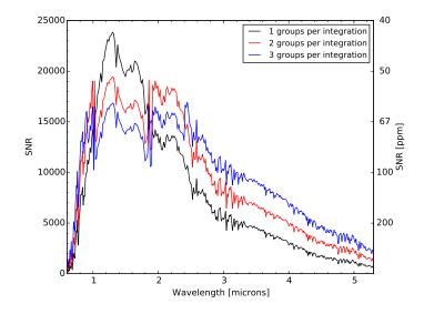
Figure 6. SNR of a NIRSpec observation of GJ1214 with the CLEAR/PRISM configuration for one transit. Twice the transit duration is spend on baseline observations, resulting in total exposure time 3x52 min. The NEETC has been run for a PHOENIX template spectrum with  $T_{\text{eff}} = 3000$  K,  $\log(g) = 5.0$  (cgs units) and J-band magnitude 9.750. The three curves represents the SNR for ng = 1, 2 and 3. SNR does not simply scale with ng due to changes in the detector duty cycle.
