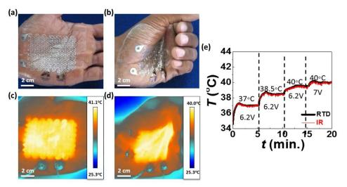
Figure 4. Skin-conformable and programmable heater. (a) & (b) An epidermal heater with on-board temperature sensor laminated on human palm under open and half-closed condition. (c) & (d) Temperature distribution without and with hand deformation. (e) The heater can heat to target temperature and hold until commanded to reach new target temperature.
