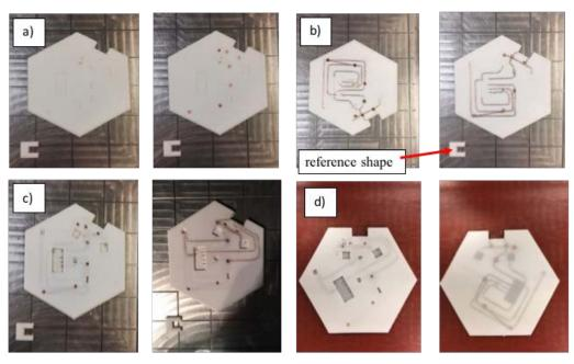
Figure 5. Wire embedding for two layer interconnection
