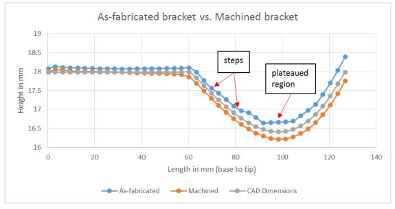
Figure 8. Bracket test print utilizing surface machining.
