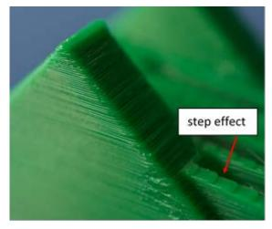
Figure 6. Example of visible layer steps.
