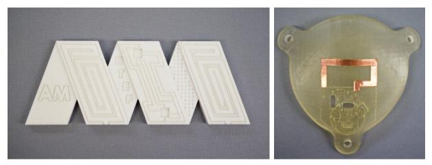
Figure 2. left) 3D printed part with machined paths, right) a part showing embedded foil and micromachined paths.
