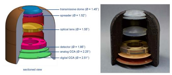
Figure 4. Left) Drawing of missile seeker, and right) completed part.
