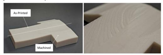
Figure 7. Bracket test print utilizing surface machining.
