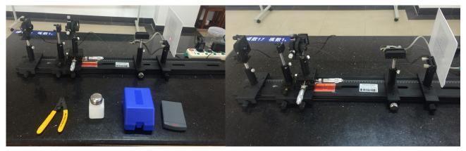
Fig. 10 Experimental setup on power coupling from free-space LD to SMF.
