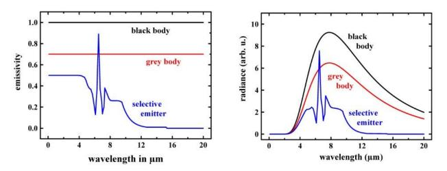
Fig. 2: Emissivities (left) and resulting radiance spectra (right) of thermal radiation for objects of T = 373K (100 °C). The emissivity may be unity (black body), constant (grey body) or vary as a function of wavelength (selective emitter).
