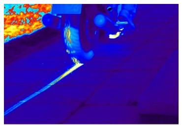
Fig. 4: Friction results in heat transfer from the tire of a motorcycle to the ground upon breaking with blocked tire.
