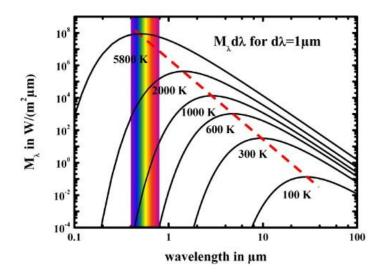
Fig. 1: Excitance spectra of black body radiation for different temperatures. For objects with typical temperatures below 2000K, the emission is predominantly in the thermal IR range between 1µm and around 20µm wavelength. The dotted line connects all maxima and visualizes Wien's displacement law.
