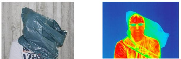
Figure 8: Plastic bags are partially transparent to IR radiation (which may also be quantified using IR spectroscopy)
