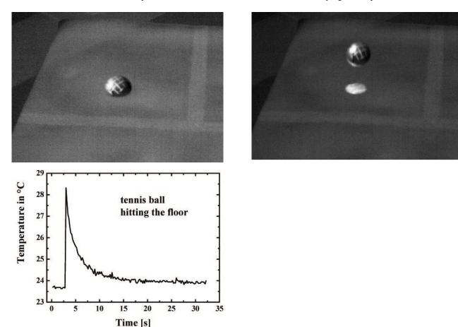
Fig. 14: Two snapshots of a high speed IR imaging sequence of a tennis ball hitting the floor and shortly afterwards while leaving it again as well as a plot of maximum temperature of the contact spot on the floor versus time.
