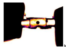
Fig. 9 A graphite tube (length = 3 cm) with a small hole (diameter = 2 mm) serves as cavity, used to record IR images while studying the transition from emission to absorption. The tube can be heated by holding its ends between fingers (a) or cooled (b) by attaching the ends to ice cubes.
