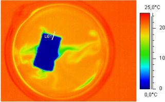
Fig. 6: An ice cube moving in room temperature water observed from above does nicely visualize convective heat transfer
