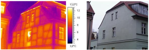
Fig. 12: Half-timbered structures of a house which are hidden behind plaster.
