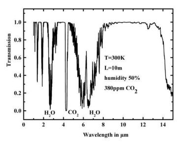
Figure 3. Atmospheric transmission (low resolution) for a standard atmosphere at T=300 K, a path length of 10 m,  $CO_2$  concentration of 380 ppm and 50% relative humidity.
