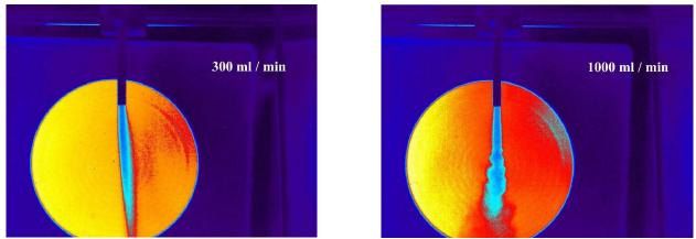
Fig. 10 Raw data of detected CO<sub>2</sub> flows of 300 ml/min and 1000 ml/min. The MW IR camera was operated with an uncooled narrow band filter in front of a black body emitter operated at T = 50 °C.
