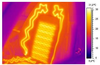
Fig. 11: Visualization of proper operation of a front seat heating system in a car.
