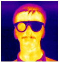
Fig. 7: Special glasses made from glass and NaCl visualize the different optical material properties in the VIS and IR.
