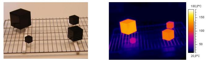
Fig. 5: Cooling of cubes of various sizes which were homogeneously heated to the same starting temperature occurs via heat transfer. The resulting law of cooling leads to faster cooling of small objects.
