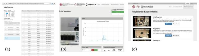
Fig. 3 Important features on RemoteLab platform. (a) Booking system for reservation of timeslots. (b) Main experiment page for controlling and monitoring the setup, as well as display and handling of collected data. (c) Collection of introductory videos for various experiment setups.
