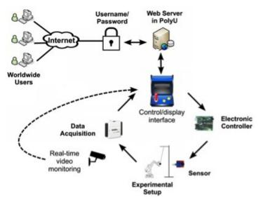
Fig. 1 Schematic diagram showing the concept of real-time, remote-access laboratory experiment platform.
