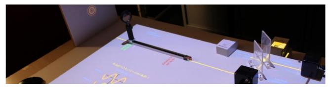
Figure 8. Simulation and augmentation of a Michelson Interferometer experiment. Physical and digital content are merged in a unique seamless environment
