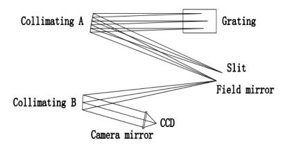
Figure 4. The optical system of spectrograph
