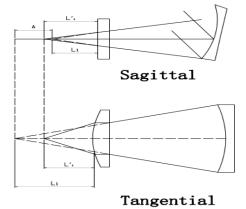
Figure 3. The theories of cylindrical lens optimize astigmatism
