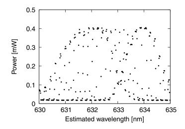
FIGURE 6: HeNe spectra as measured by grating setup. These peaks have a FWHM of less than 0.1 nm, suggesting that these features are artifacts, as the grating cannot resolve details beyond 0.1 nm, the theoretical resolution limit.
