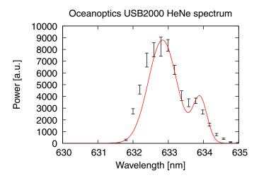
FIGURE 5: HeNe laser spectrum as measured by the Oceanoptics USB4000 spectrometer, fitted to a bi-Gaussian. Error-bars are the computed standard deviation at each point.
