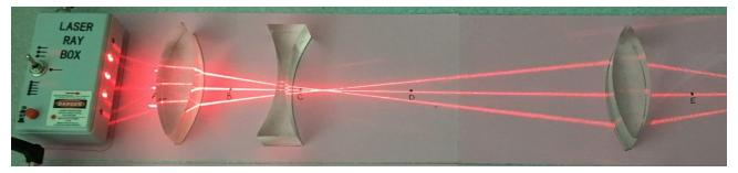
Figure 1. Laser ray box with converging and diverging lenses. Here points A, B, C, D, and E represent points where students could identify parallel, converging, or diverging rays and wavefronts, positive, negative, or zero vergence, and real, virtual or distant objects and images for each lens.
