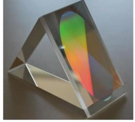
Fig. 5. GRISM bond with ALD-coated grating at the outer surface
