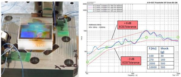
**Fig. 8.** Set-up for shock test (left) and corresponding z-axis acceleration vs. frequency diagram (right) *C. Alignment*
