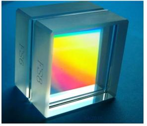
Fig. 6. Prism-grating-prism type bond using prism dummies of plane-parallel shape
