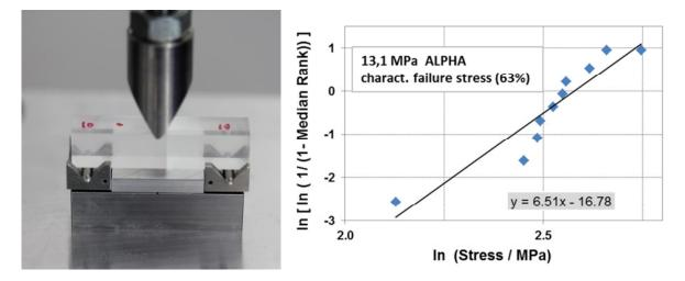
Fig. 7. Set-up for 3-point bending test (left) and Weibull analysis of bond strength values (right)
