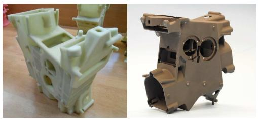
Fig. 2. The Spectrolite housing. On the left the wax model and on right the final (black anodized) structure.
