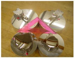
Fig. 3. The four Spectrolite mirrors after manufacturing
