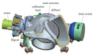
Fig. 7. Optic-Structure of the calibration unit
