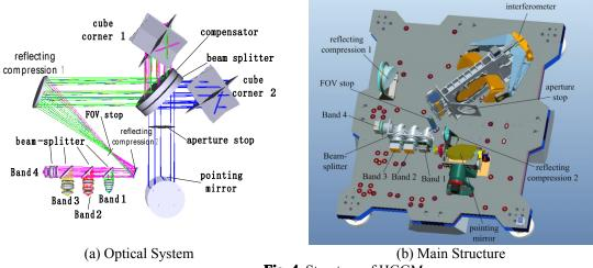
Fig. 4. Structure of HGGM
