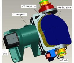
Fig. 6. Optic-Structure of the pointing mirror mechanism
