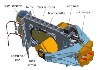
Fig. 5. Optic-Structure of the interferometer
