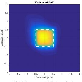
Fig. 9 Non-symmetric PSF of one pixel
