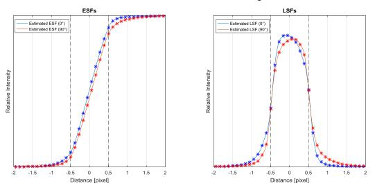
Fig. 8 Non-symmetric signal from KE measurements (left: ESF, right: LSF; for two scanning directions)
