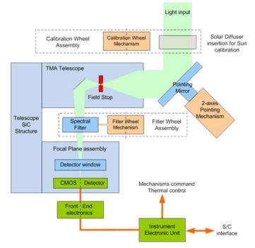
Fig. 3: Functional architecture of the GOCI-II instrument
