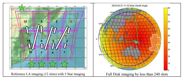
Fig. 5: Two imaging modes are available: Local area acquisition and Full Disk acquisition
