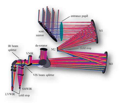
Fig. 4 METimage optical design.
