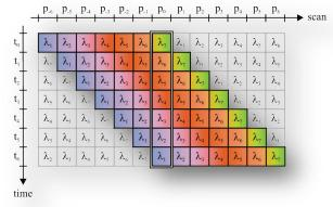
Fig. 2 METimage scanning principle, illustrating the sequential measurement of a pixel p within 1 scan over time t.
