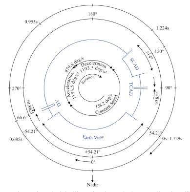
Fig. 3 METimage observation principle, illustrating the Earth view as well as the calibration views.
