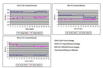
Fig. 1. TID up to 30Krads of XC2C256 CoolRunner<sup>™</sup>-II CPLD and OPA354.
