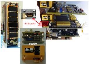
Fig. 1. View of the OPTOS satellite, distributed architecture, optical diffuse cavity and a complete OBCOM module.
