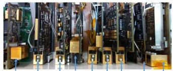
TPA EPH EPS ADCS FIBOS GMR ODM\_MGM EGSE + BATTERY Fig. 3. OBCOM distribution in OPTOS satellite.
