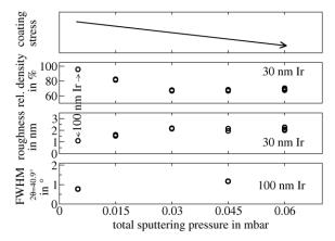
Fig. 4. Properties of the iridium thin films as a function of the total sputtering pressure [34].
