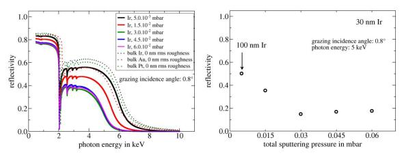
**Fig. 5.** Calculated X-ray reflectivity of the Ir thin films with density and rms surface roughness of Fig. 4. Calculations obtained from [22, 23] using a grazing incidence angle of 0.8°. Left: Plot as a function of the photon energy including a comparison to the X-ray reflectivity of Ir, Au and Pt bulk materials with assumed rms surface roughness of 0 nm. Right: Plot as a function of the total sputtering pressure at a photon energy of 5 keV.
