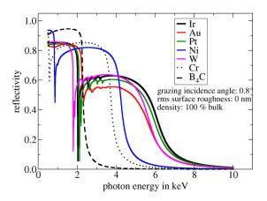
**Fig. 2.** Computed X-ray reflectivity behavior of different coating materials for a grazing incidence angle of 0.8° and assuming a bulk density and no surface roughness. Calculations obtained from [22, 23].
