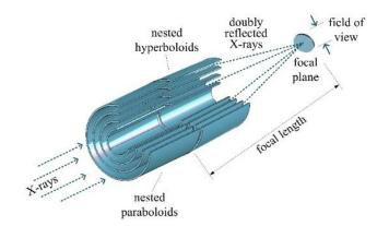
Fig. 1. Schematical representation of the principle of a segmented Wolter I type X-ray telescope [4].
