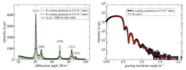
**Fig. 3.** Left: X-ray diffractogram of two 100 nm thick Ir films sputtered at  $5.0 \cdot 10^{-3}$  mbar (green) and respectively at  $4.5 \cdot 10^{-2}$  mbar (black), and calculated X-ray diffraction peaks of cubic face centered (fcc) Ir from the Powder Diffraction File 03-065-1686 [31, 30] (red). Right: Grazing incidence X-ray reflectometry measurement data (circles) of a X-ray mirror with a 30 nm thick Ir film coated at  $4.5 \cdot 10^{-2}$  mbar and corresponding fit curve (red line).
