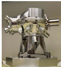
**Fig. 6.** QM calibration units. Left: Full aperture solar diffusor hatch. Right: The on-board calibration assembly including the two calibration spheres.
