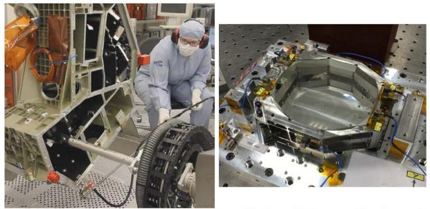
Fig. 5. Left: Final ISO5 cleaning of the IOU. Right: prism qualification model after successful environmental qualification at IABG.
