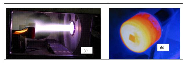
Fig. 5: Photograph of (a) the Plasma hitting the center of the probe with the FBG, the second adjacent is the heat flux probe, and (b) Image provided by the IR camera
