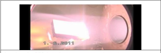
Fig. 7: Picture of the C-SiC with the Fibers and Thermocouples during the Wind Tunnel test at DLR
