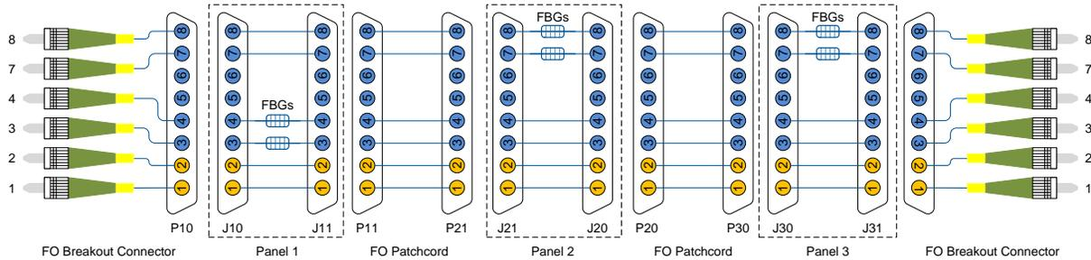
**Figure 5: Illustration of the planned harness shown for the panel internal wiring and the patchcord connections.**
