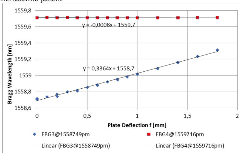
Figure 4: Measurement results of the four-point bending test for the pure FBG glued onto the plate (blue curve) and for the FBG mounted inside the special designed transducer (red curve).
