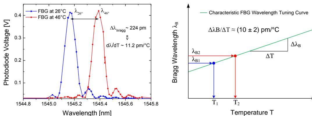
**Figure 2: Measurement of an FBG spectrum at two different temperatures (left) and a scheme of a characteristic Bragg Wavelength vs. Temperature tuning curve (right).**
