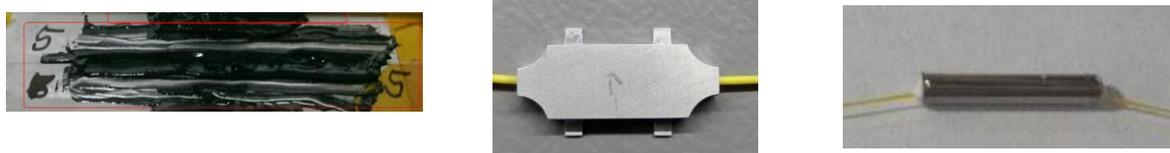
Figure 3: Left: pure FBG glued onto panel plate. Middle: Feedthrough based transducer. Right: Capillary based transducer.
