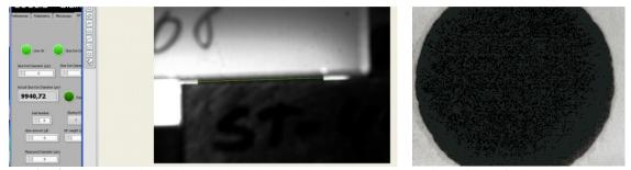
Fig. 4: Edge detection during bonding process and detailed close-up inspection of a bonding pad
