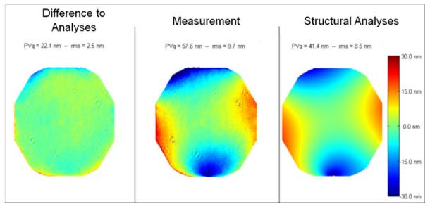
Fig. 7: Gravity induced SFE measurement and initial analysis results
