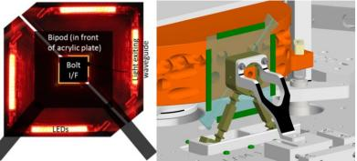
Fig. 10: Background illumination system for bolt type bonding interfaces
