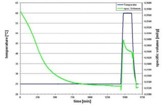
Fig. 5: Specific volume change and temperature profile over time during adhesive curing (measured by mercury-volume dilatometry
