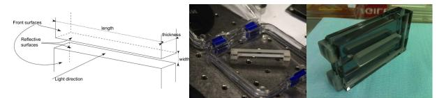
**Fig. 5**: a) Left: General setup of a slit homogenizer (SH). b) Middle: SH prototype for Concept A (photo courtesy of Airbus DS) c) Right: SH prototype for Concept B (photo courtesy of WinLight)
