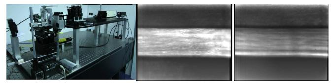
**Fig. 6**: a) Left: Test setup for SH performance testing (photo courtesy of ITO). b) Middle: SH response (image of slit exit) to homogeneous illumination. c) Right: SH response to half-slit (knife-edge) illumination.
