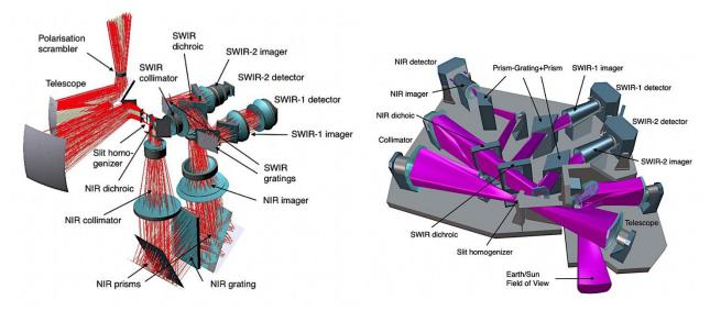
**Fig. 1:** Designs concepts for the CarbonSat instrument resulting from the industrial Phase A/B1 studies. Concept A on the left was developed by the consortium led by Airbus DS, Concept B on the right by OHB/Thales.
