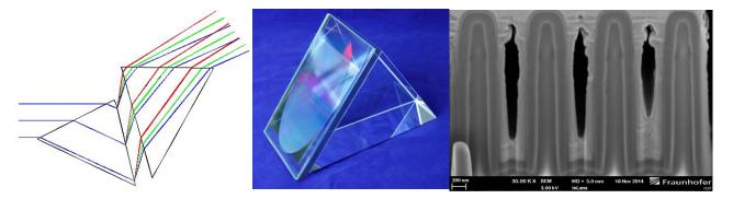
**Fig. 3**: a) Left: Light path though the prism-grating-prism (PG+P) assembly. b) Middle: The bonded prism grating prototype assembly (photo courtesy of IOF). c) Right: SEM image of the binary sub-micron structure on the surface of the grating substrate.
