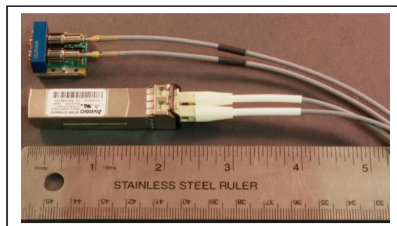
Fig. 5. Size comparison of Glenair 2-fiber transceiver with commercial datacom SFP pluggable transceiver.
