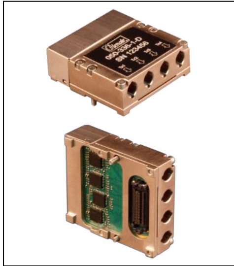
Fig. 3. PCB-mountable quad-output transmitter unit: Top view (upper) and bottom view (lower).
