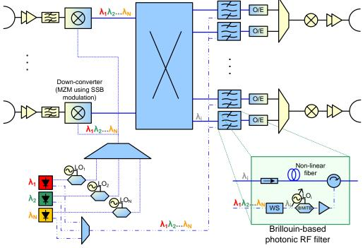
Fig. 8. Photonic payload architecture integrating Brillouin-based photonic RF filtering
