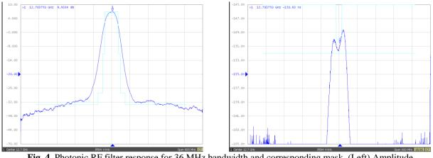
**Fig. 4.** Photonic RF filter response for 36 MHz bandwidth and corresponding mask. (Left) Amplitude. (Right): Group delay.
