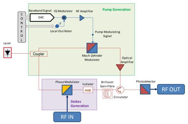
Fig. 1. Photonic RF filtering architecture
