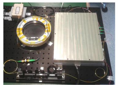
Fig. 2. Photonic RF filtering demonstrator
