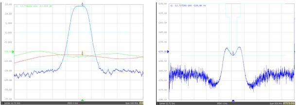
**Fig. 6.** Photonic RF filter response for 72 MHz bandwidth and corresponding mask. (Left) Amplitude. (Right): Group delay.
