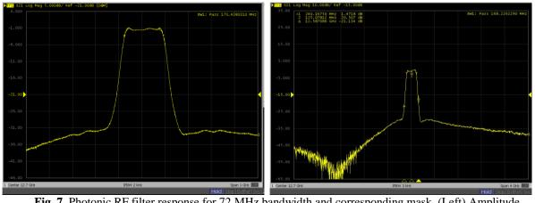
**Fig. 7.** Photonic RF filter response for 72 MHz bandwidth and corresponding mask. (Left) Amplitude. (Right): Group delay.
