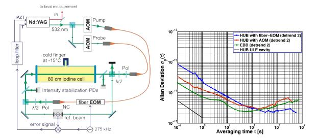
Fig. 1. Left: Schematic of the laboratory setup of the iodine frequency reference at the Humboldt-University Berlin [6]. Right: Frequency stability of iodine-based frequency references [6]. The blue curve corresponds to the HUB laboratory setup as presented in section I using a fiber EOM for phase modulation. The red curve corresponds to a similar setup using an AOM for phase modulation. The green curve shows the frequency stability of the EBB setup as detailed n section II.
