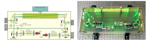
**Fig. 2.** Schematic and photograph of the spectroscopy setup developed on elegant breadboard level. The baseplate has dimensions of 25 cm x 55 cm [6].
