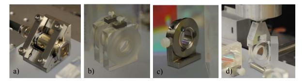
**Fig. 4.** Detail photographs of the fiber collimator with Invar mount and polarizer (a), the pair of wedged glass plates (Risley prism pair) with all-glass mounts (b), the waveplate with titanium mount (c), and a lense mounting during integration process (d).
