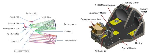
Fig. 1: TMA telescope optical layout (left panel) and 3-D view of the telescope breadboard (right panel)
