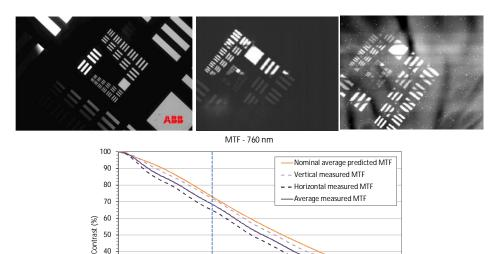
**Fig. 4:** VNIR, (top left) SWIR (top center) and M/LWIR (top right) images of a USAF resolution chart obtained with the Multi-Spectral Imager Breadboard. Raw uncalibrated and uncorrected data. The MTF measured at 760 nm in the VNIR channel is shown in the bottom panel.
