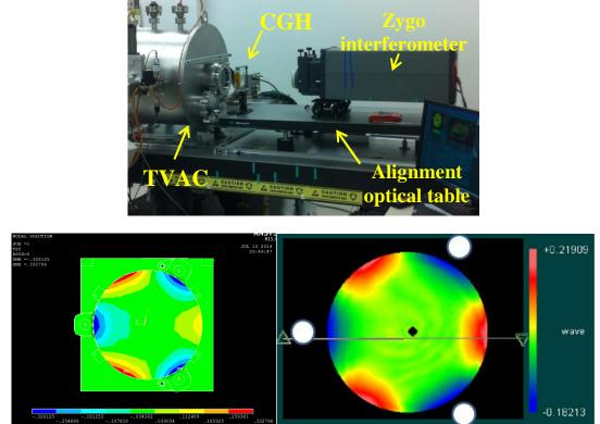
**Fig. 5:** The differential surface deformation for the tertiary mirror between a temperature of 22.5 °C and 17 °C simulated in the STOP analysis (bottom left) are compared to the laboratory measurement (bottom right). The power and astigmatism terms are removed from both results. The test setup is shown in the top panel.
