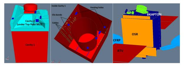
**Fig. 5.** EDRS-C inside and outside materials
