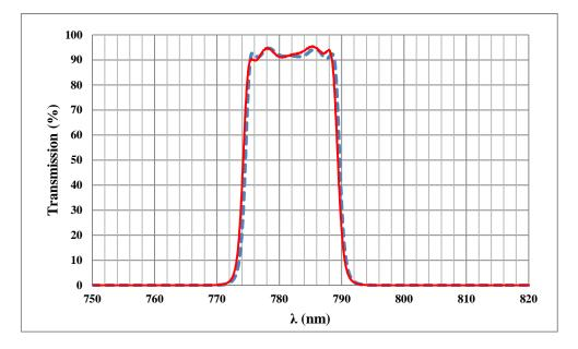
Fig. 6. Comparison between theoretical (dashed line) and experimental (solid line) transmission of the VIS Filter 2.
