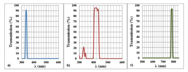
**Fig. 4.** Transmission spectra of the UV-VIS deposited filters: UV Filter (a), VIS Filter 1 (b) and VIS Filter 2 (c).
