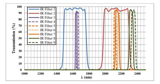
Fig. 5. Transmission spectra of the IR deposited filters.
