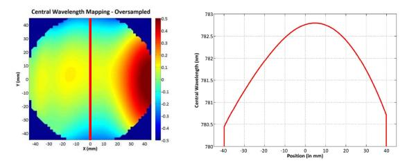
**Fig. 8.** Result of the spectral uniformity measurement on the filter side of the VIS Filter 3 (Cartography and shape of the central wavelength of the filter along the red line).
