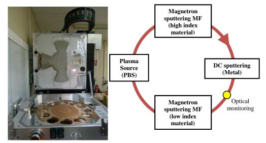
Fig. 1. HELIOS deposition process chamber. Proc. of SPIE Vol. 10563 1056306-2
