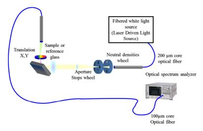
Fig. 2. Spectral uniformity measurements set up.
