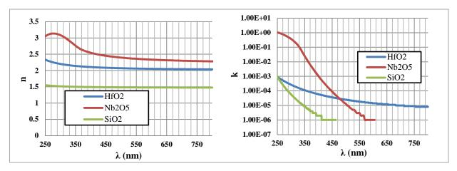
Fig. 3. Refractive indices (n) and extinction coefficients (k) of the materials deposited with the HELIOS System.
