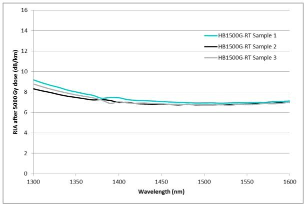
Fig. 2. RIA over operational wavelength range of HB1500G-RT samples after a total dose of 5000Gy.
