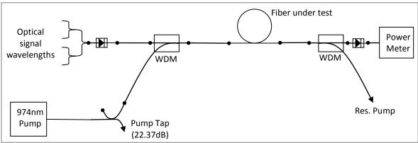
Fig. 1. Single pump EDFA photo-anneal set up
