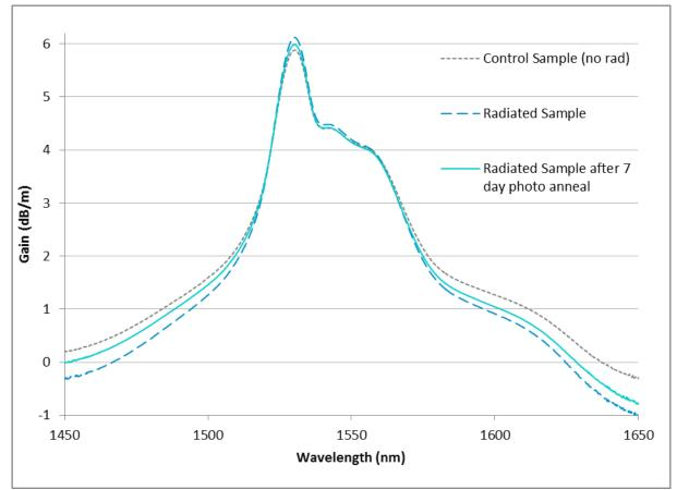
Fig. 5. A-3 fiber gain spectra before irradiation, after irradiation (200Gy) and after a 7 day photo anneal.
