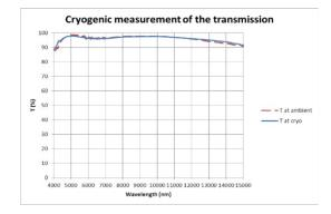
On this measured curve, we have superimposed the theoretical expected curves (dashed lines) and the measured one (solid lines, red for transmittance and blue for reflectance).
