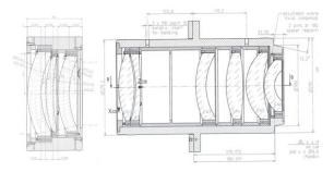
Fig. 3: EMIR collimator (on left) and camera (on right)
