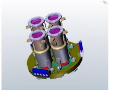
After being spectrally separated and collimated, the NIR/IR optical beams reach the cold optics, which are located inside a common cryostat.
