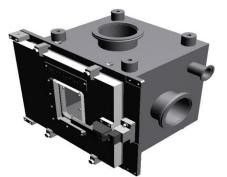
The deformation is measured in ambient conditions, but a dedicated chamber is being prepared to allow a measurement under vacuum to assess the effect of environment.
