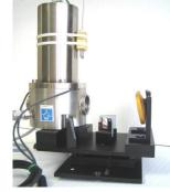
The Dewar can be adapted onto our  $12^{\circ}$  absolute reflectance accessory. Connected to a **controller**, it can also allow heating the sample in high temperature conditions (up 350°C) to allow measurements in good conditions. The Dewar is equipped with ZnSe windows which are heated to avoid condensation. The cell can be brought to vacuum using a convenient connection to a pumping system. It can also be used under dry nitrogen for simpler configuration.
