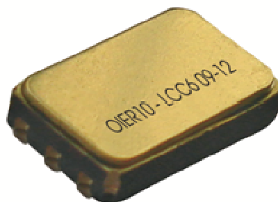
Figure 1: Optoi's optocoupler coded OIER10, mounted in a LCC package with 6 pins
