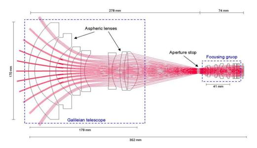
Fig. 3. The 3MI VNIR module optical design
