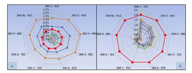
**Fig. 5.** Typical 3MI AR coating performances optimised to deliver minimum polarisation sensitivity (a) as well as minimum de-phasing (b) at component level. The red line shows the target performance for this run. The coloured lines indicate the coating performance for the various lens elements at a typically large AOI.
