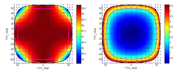
**Fig. 6.** Typical e2e polarisation sensitivity simulation for a 3MI polarised channel (left) and a 3MI un-polarised channel (right). Performances degrade for increasing field angles given the increased AOIs on the AR coatings.
