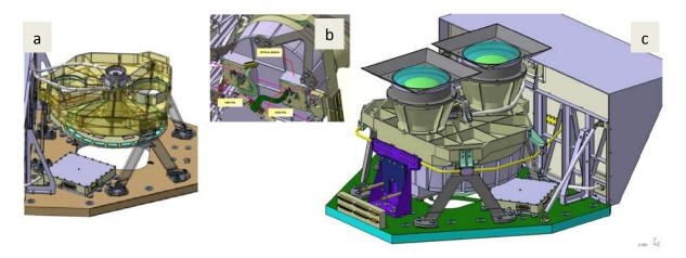
Fig. 1. Key elements of the 3MI Instrument OMU: (a) filter wheel mechanism and disk, (b) focal plane assemblies, and (c) the two optical heads and the thermal hardware.
