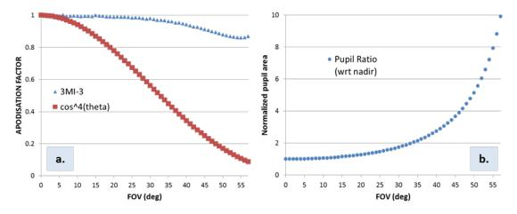
**Fig. 4.** (a) Typical 3MI (blue curve) irradiance variation over the focal plan assuming a uniform scene, (b) typical variation of the effective pupil over the FOV of 3MI
