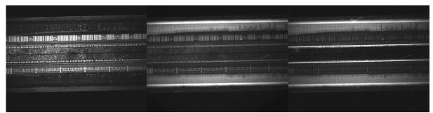
**Fig. 6.** PLEIADES detector from left to right: 450 nm excitation wavelength filter (1s), 550 nm filter (20s) and 650 nm filter (45s). Dark subtracted but no Flat correction.
