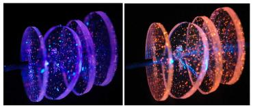
**Fig. 3.** Nanoparticles in MAPSIL213 irradiated respectively from left to right with 365 nm and 450 nm excitation sources. On the left, nanoparticles have a low emission due to their weak absorbance at 365 nm. On the right the excitation is optimum. We can also see the emission of textile particles due to the brightener included in washing powders.
