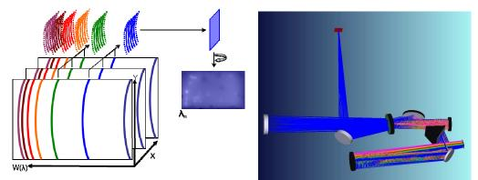
Fig. 8a. Image reconstruction. Fig. 8b. 3D view of the beams for 5 points in the vertical field of view and their corresponding projections for 5 different wavelengths
