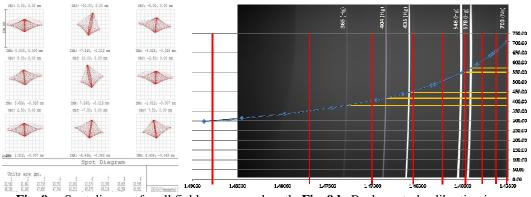
Fig. 9 a. Spot diagram for all fields, one wavelength. Fig. 9 b. Real spectral calibration image
