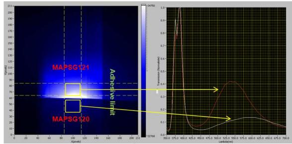
Fig. 10 a. Picture at 550\_nm extracted from the hyperspectral cube. Fig. 10 b. Spectrum extracted in the other direction from the two yellow rectangles
