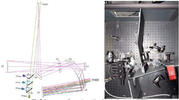
Fig. 7. Spectrometer: Ray tracing and bench in development at CNES
