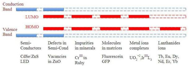
Fig. 1. The luminescence is associated to the transition of an electron from the Conduction to the Valence band in semiconductors[3], from the LUMO to the HOMO levels in small emitters [2] and between magnetic sub-levels of the LUMO for Lanthanides[4]
