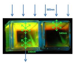
**Fig. 2.** Transmission of fluorescein in aqueous solution for high concentration (right) and low concentration (left). On the right cell, the absorption due to the fluorescein is strong and there is a saturation of the fluorescence. On the left cell, the concentration is optimized to balance absorption through the overall cell. The yield is better for this lower concentration.
