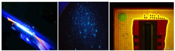
**Fig. 4a.** Picture of the rear side of a mirror taken with a classic reflex camera in visible light (excitation 365 nm). The red fluorescence corresponds to the primer and the blue color to the adhesive.
