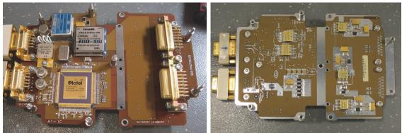
Figure 5: Front and back view of the HERMOD PFM PCB just after the components being mounted.
