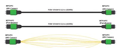
Figure 7: Different test vehicles used for on-ground evaluation testing of the optical assembly
