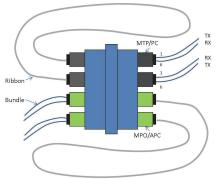
Figure 4 Design of the HERMOD optical assembly including the 4 channels.
