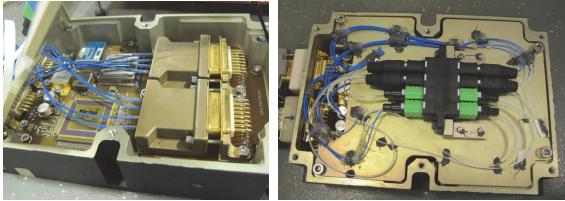
Figure 6: Electronics and SIOS modules (left), optical assembly and fiber routing on the upper layer (right).
