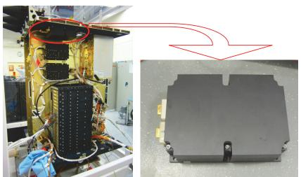
Figure 8: HERMOD PFM payload before(right) and after (left) integration on Proba-V platform.
