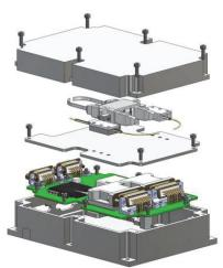
Figure 3 Exploded view of HERMOD box including the optical (upper) and electronic (lower) layers.
