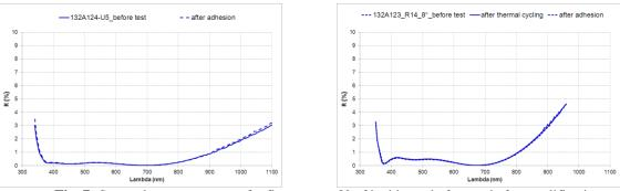
Fig. 7: Spectral measurements of reflectance at 8° of incidence before and after qualification tests
