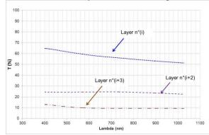
Fig.5. In-situ measurements of transmittance under vacuum over a broad spectral range
