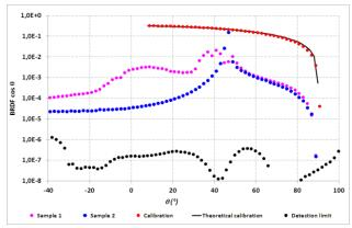
Fig. 12: Scattering measurement of 2 samples with different roughnesses,  $\lambda = 600$  nm at 50° of incidence
