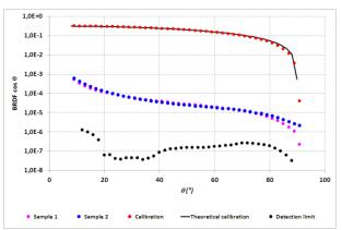
Fig. 11: Scattering measurement of 2 samples with different roughnesses,  $\lambda = 600$  nm at 0° of incidence
