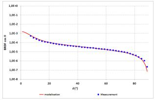
**Fig. 13:** BRDF measured (black dots) compared with modelization (red curve) of scattering losses of absorbing optical coating – Unpolarized illumination light at 650 nm wavelength under normal incidence
