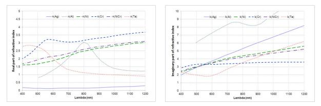
Fig.1. Refractive indices of metals as a function of wavelength
