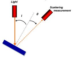
**Fig. 10:** Definition of angles of incidence (i) and scattering  $(\theta)$
