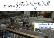
Fig.4. In-situ broadband optical monitoring connected to 14 m<sup>3</sup> PACA2M coating chamber
