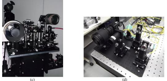
Fig. 3. Photo of the optical system setup: c. receiver module; d. transmitter module
