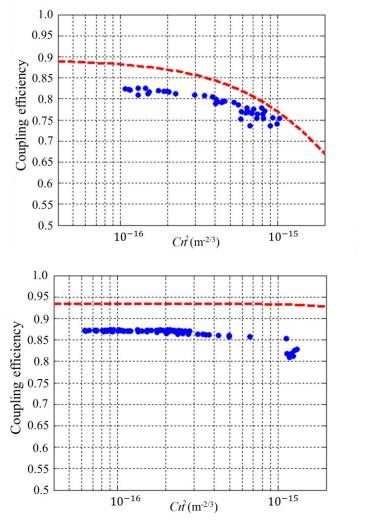
Fig. 6. The coupling efficiency of laser beam to MMF The core radius of the MMF (top:  $200 \mu$ , bottom:  $600\mu$ )
