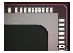
**Fig. 11** Picture of an ARC coated EUROCIS imager die. The dark region is the AR coated area, the light region is uncoated silicon. The top and right of the picture show the uncoated bond pads.
