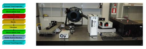
Fig. 13 Characterization sequence (left) and optical setup for EUROCIS (right).
