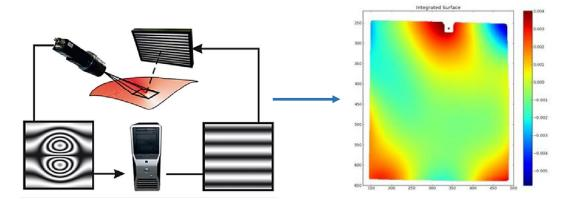
**Fig. 5.** Schematic view of the deflectometer to measure deformations in the glass. The picture on the right is a real measurement of a deformed surface due to glue influence.
