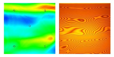
**Fig. 4.** Comparison of glass thickness measured by optical sensor (left) with double beam interference pattern (right) using sodium light. This glass has a peak-to-valley thickness variation of 10μm.
