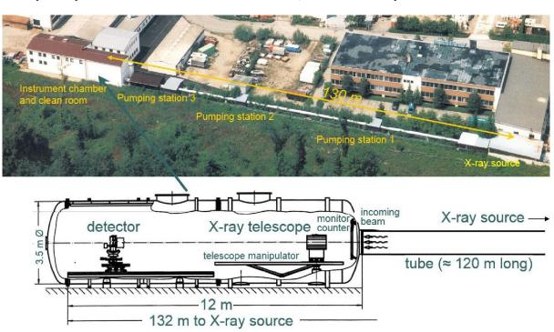
**Fig. 7.** PANTER X-ray testing facility. The lower panel shows a detailed schematic view of the instrument chamber.
