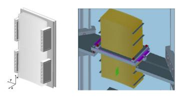
Fig. 6. Model of current 8-point mounting system (left) and new central based integration system (right)
