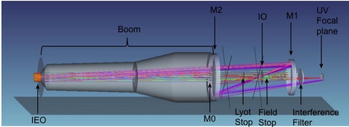
Fig. 1 - Schematic layout of METIS UV path.
