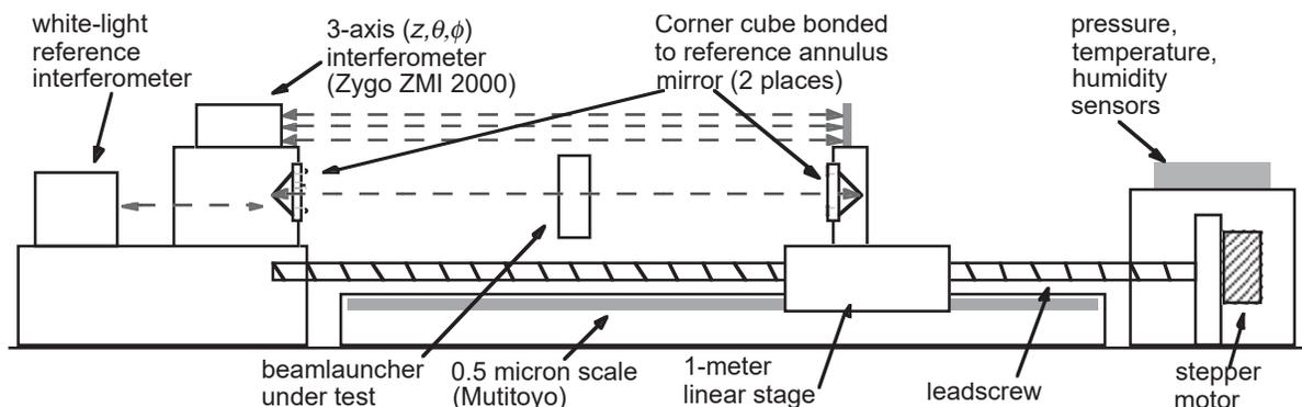
Figure 10: Layout of absolute calibration stand.
