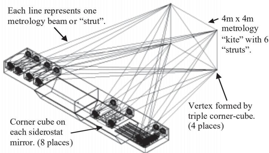
Figure 2: External metrology used to monitor the geometry of SIM to  $\sim 100$  pm. *Geometry* means the precise lengths, relative directions and positions of  $D_1$ ,  $D_2$ ,  $D_3$ , the baseline vectors of the three interferometers (science and two reference).
