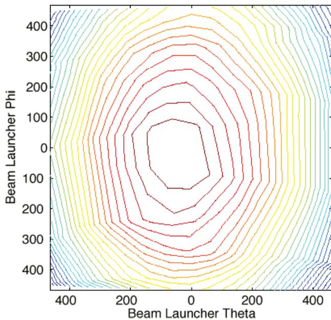
Figure 12: phasemeter output ( $L$ ) as a function of beamlauncher elevation and azimuth angle. Each contour is 0.002 cycles or 1.3 nm. The central region, near perfect alignment, has a *maximum* in  $L$ .  $L \approx 2$  m. Theta, phi: arbitrary units.
