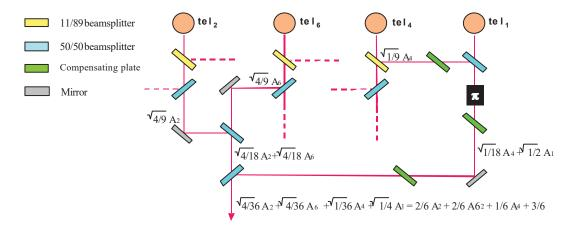
Figure 5 Beam-combining principle of the 3-GAC nulling interferometer
