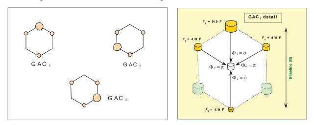
Figure 1 The Laurance nulling space interferometer consists of 6 equal size telescopes flying in a hexagonal formation, with the beam-combiner in the centre.
