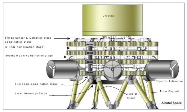
Figure 11 Beam-combiner mechanical architecture
