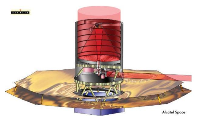
Figure 4 Telescope thermo-mecanical concept
