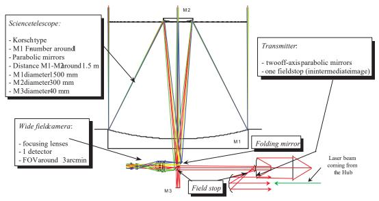
Figure 3 Telescope collector optical concept
