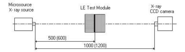
Fig. 5: Arrangement of the X-ray tests of the improved Schmidt test module. The indicated measures are in mm.
