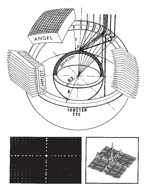
**Fig. 1**: Arrangement of lobster-eye X-ray lenses based on Schmidt and Angel geometry. Bottom left: real optical image of distant point-like source, bottom right: computer ray-tracing for a point-like source.
