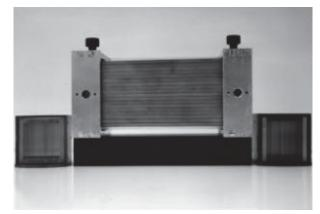
Fig. 3: Prototypes of L-shaped Angel (left) and mini (23 x 23 mm plates) Schmidt (right) X-ray telescopes
