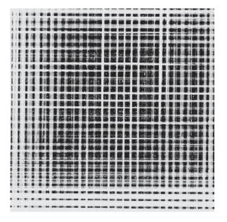
**Fig. 6**: The X-ray shadow gram of the LES module showing the 100 micron thick gold plated flats and approx. 300 (500) micron spaces separating them (and also confirming the high optical quality of used flats).
