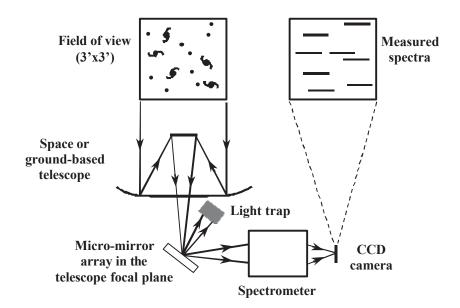
Fig. 1: Principle of Multi-Object Spectrograph with a Multi-Mirror Array for NGST.
