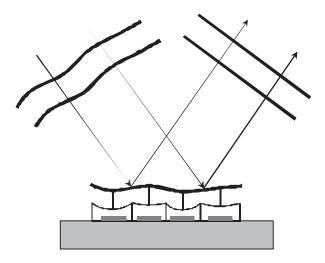
Fig. 6: Principle of wave front correction using a Micro-Deformable Mirror (MDM).
