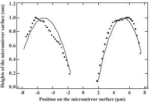
Fig. 4: Reconstruction of the micro-mirror surface along the central line of mirror 1 of the third row of micro-mirrors in Fig. 4, obtained by integration of measured slopes Parabolic approximation is superimposed.
