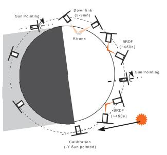
1 radiometric calibration using diffusers, illuminated by Figure 2 : Typical operations during an orbit with downlink
