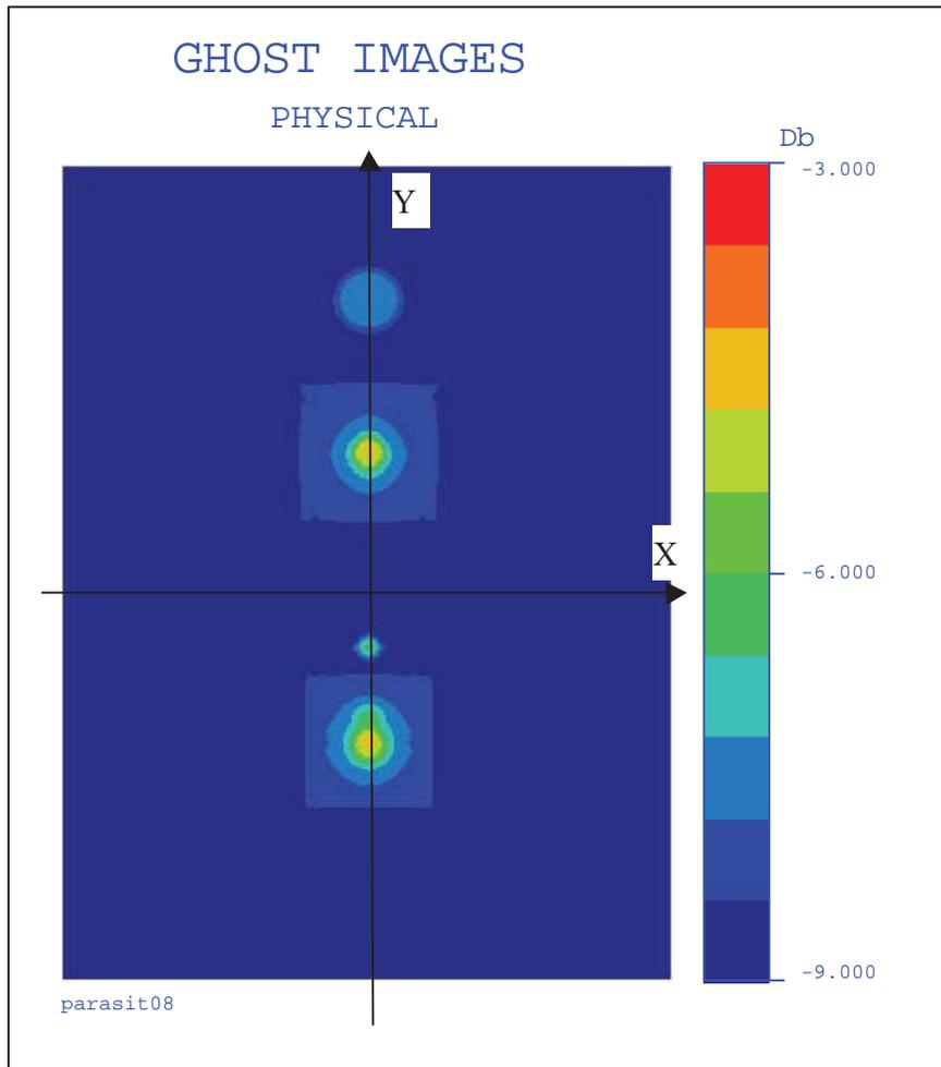
Fig. IV : Physical analysis (PSF) of the ghost images of Fig I.
