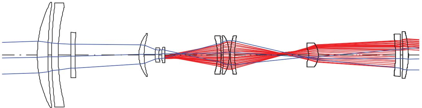
Fig. I : Example of stray light (in red) corresponding to a direct image
