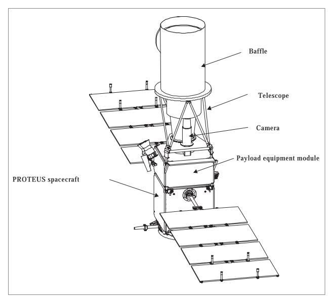
Figure 11 COROT instrument on the Proteus spacecraft
