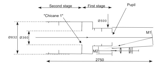
Figure 8 Optimal locations for baffle chicanes
