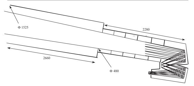
Figure 5 Baffling concept for a TMA telescope
