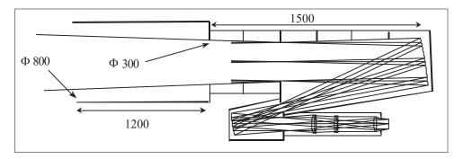
Figure 6 Baffling concept for the afocal telescope – imaging camera design
